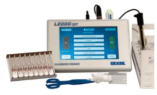
If waiting for laboratory results for surface wipes is not an option, the L2000DXT system can provide on-the-spot screening in just a few easy steps with results in less than 10 minutes. This test method requires wiping an area 1000 cm $^2$ ; results are provided in  $\mu g$  PCB/100 cm $^2$ .
